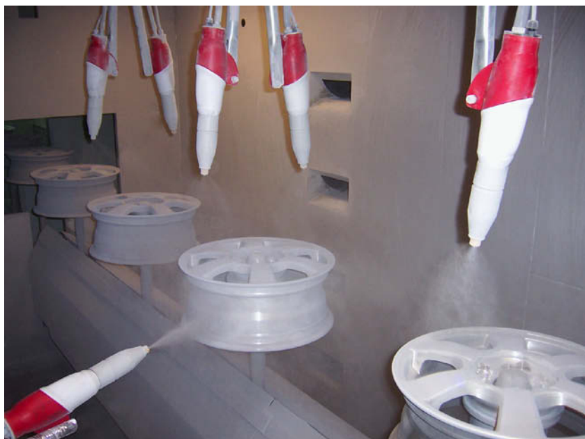
Primer coating on aluminium wheels with Auto-Mach-Jet sprayer.
